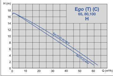
High performance wet rotor circulation pump with flanged or threaded connection, motor with permanent magnets and built-in electronic controller.
