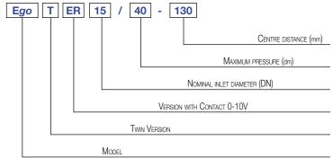
High performance wet-rotor circulation pump with threaded connection, motor with permanent magnets and built-in electronic controller.
