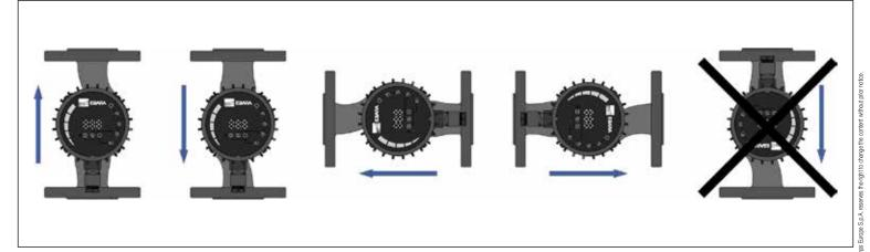
All Ego circulators should be installed with the motor shaft in full horizontal position, as shown in the figure above (example valid for all models). The power cord should never be positioned upwards (it may facilitate water inflow into the terminal box): in these cases, you should rotate the electronic unit or pump's body (please refer to the manual).
